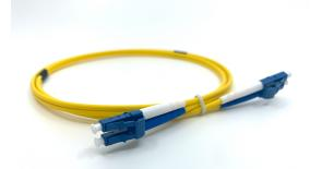
The duplex fiber patch cord is OS2 with 3 mm jacket. It is LSZH rated and its terminated with LC fiber optic connector on both ends.
